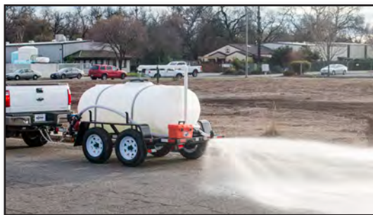
The rear mounted water nozzle creates a 16' wide pattern
