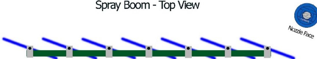
If the nozzles are aligned parallel to the structure the spray patterns would intersect and cause streaks. This image slightly exaggerates the proper pattern alignment. With threaded style nozzle caps/bodies this angle needs to be adjusted manually. Quick connect, (1/4 turn), nozzle caps/bodies come pre-aligned.
